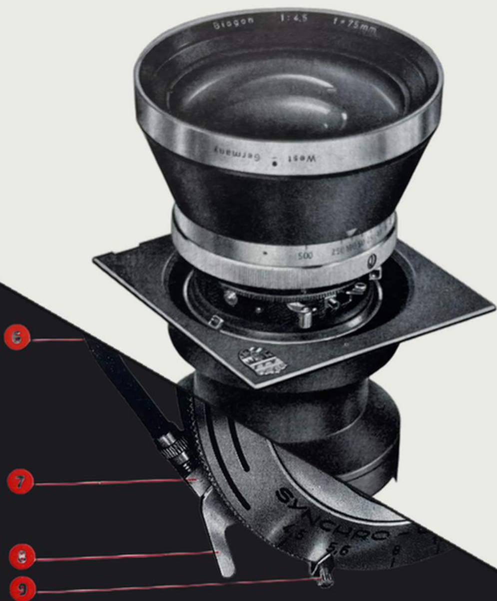
Fig. 104. Synchro Compur II: 1. Flash terminal, 2. Shutter cocking lever, 3. Delayed action knob, 4. Setting ring and window for shutter speed, 5. Press focusing button, 6. Synchroselection selector, 7. Release cable socket, 8. Release lever, 9. Diaphragm setting lever.
